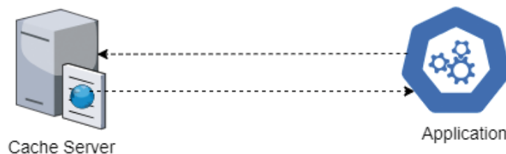
Figure 6: Data is served from the cache for subsequent requests
